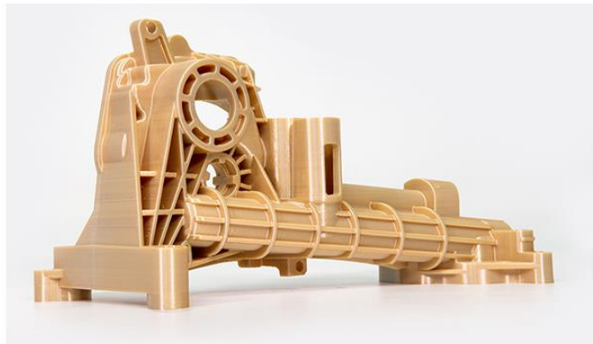
Part printed with SABIC's ULTEM™ AM9085F filament after AMS31F support material is removed
